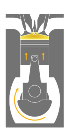
The cylinder compresses the air and fuel
