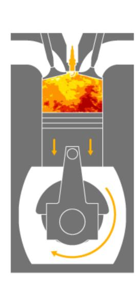
The mixture is ignited, pushing the piston down and turning the crankshaft
